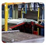
Radiators on way for pressure testing and quality control
